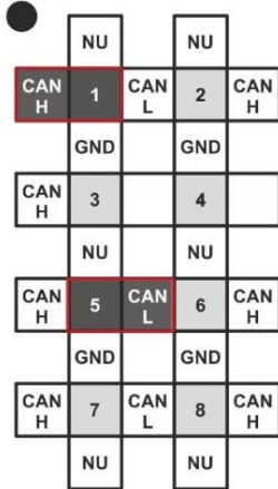
Jumper settings for Power Lite
